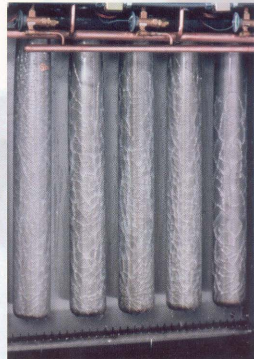
Ice is formed on both the inside and outside evaporator walls for maximum ice production.
